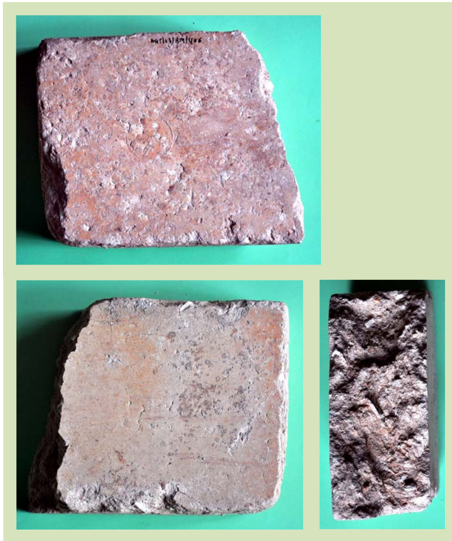
Figure 15. Machine-made fire brick. GT 03 BM 406. (ph 0880, 0882, 0885)
