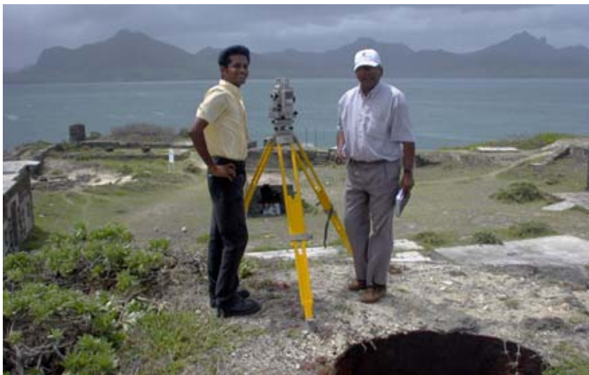
Surveyors from the Ministry of Lands and Housing making a Topographic Survey. The Sokkia Total Station is set up on the southern end of the Upper Battery. (02jv0616)
