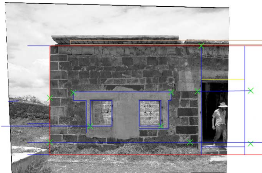
The rectified photograph is imported into AutoCAD where details from the selected elevation plane can be digitised. The green crosses are the control points used in the rectification process.
