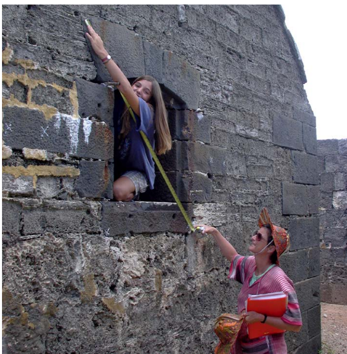
A few control points, either features or small chalk crosses, allows a photograph to be rectified so that details can be drawn in AutoCAD or traced by hand. (01jv0707)
