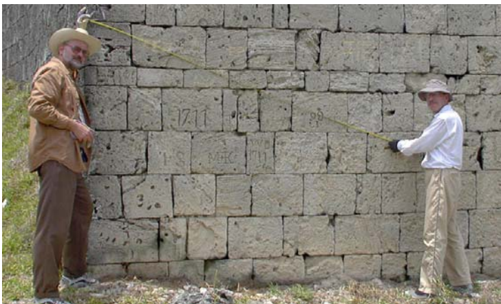
Roger and George measuring control points for photo rectification. (03jv0114)
