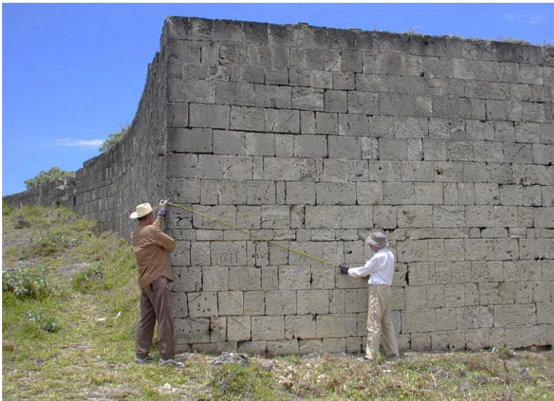
Earthwatch team members Roger and George measuring control points on the end wall of the Upper Battery for photo rectification. (03jv0113)
