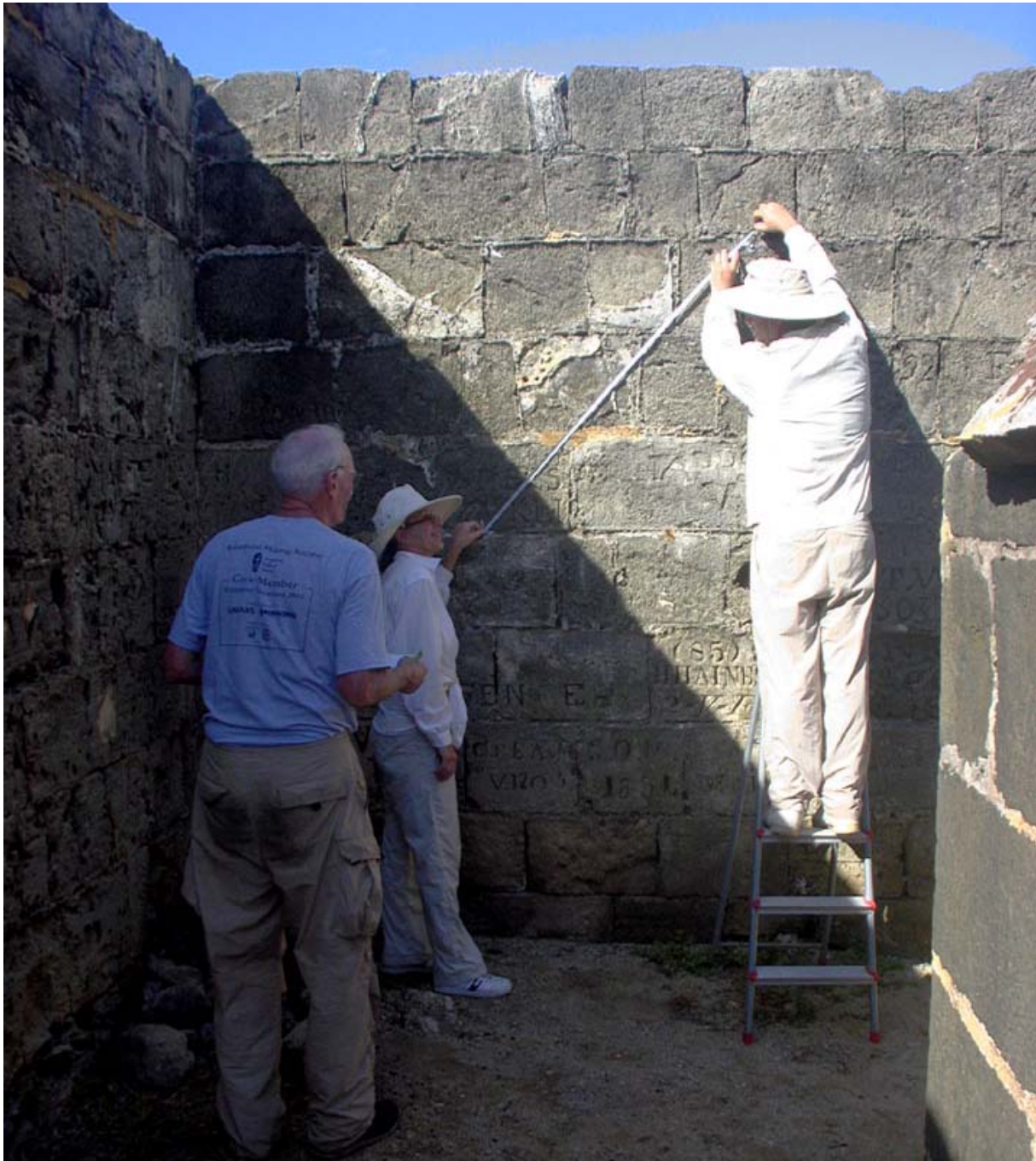
Figure 23. Rod, Rosanne and Mark measuring control points needed for the rectification of digital photos. Graffiti on the enclosure wall of the Powder House is being recorded and drawn using this technique. (04jv2111)
