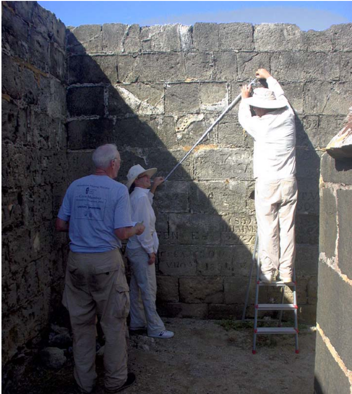
Figure 26. Rod, Rosanne and Mark measuring control points needed for the rectification of digital photos. Graffiti on the enclosure wall of the Powder House is being recorded and drawn using this technique. (04jv2111)
