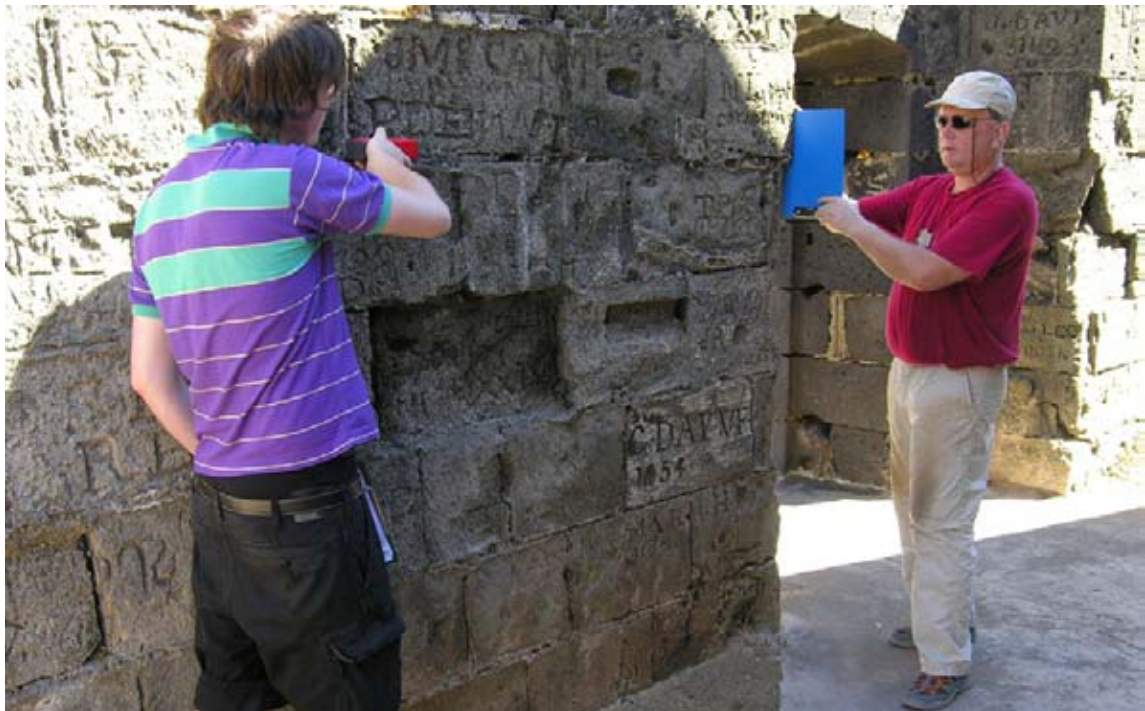
Figure 39. Owen Jones, a British postgraduate student in architecture, used his laser meter to measure control points for photorectification. (mp06nc1308)
